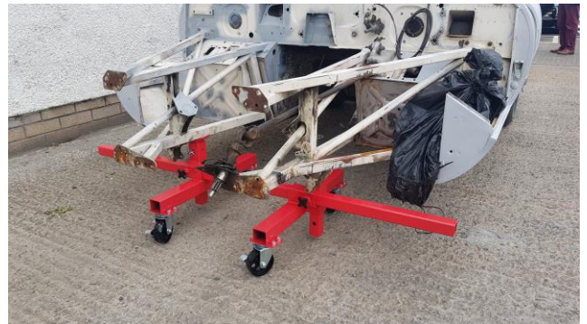
Use of one of Investor Classics' chassis dollies to manoeuvre the chassis without front wheels
