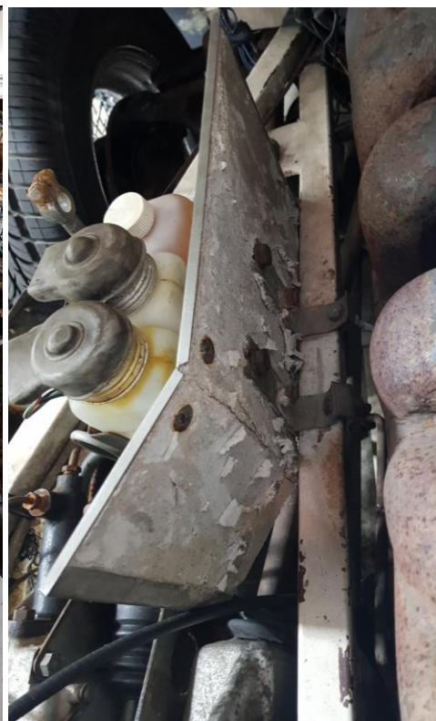
Asbestos shielding, between exhaust and brake fluid, flaking off
