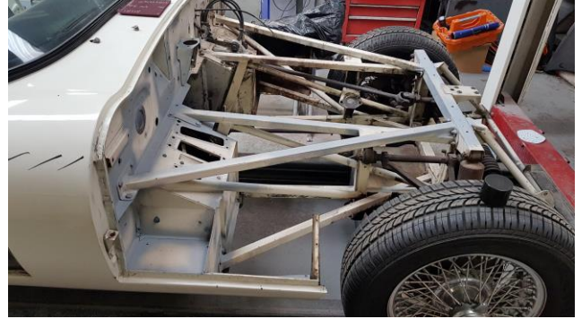
Final strip-down and treatment of surface rust prior to delivery of body to a specialist paint company
