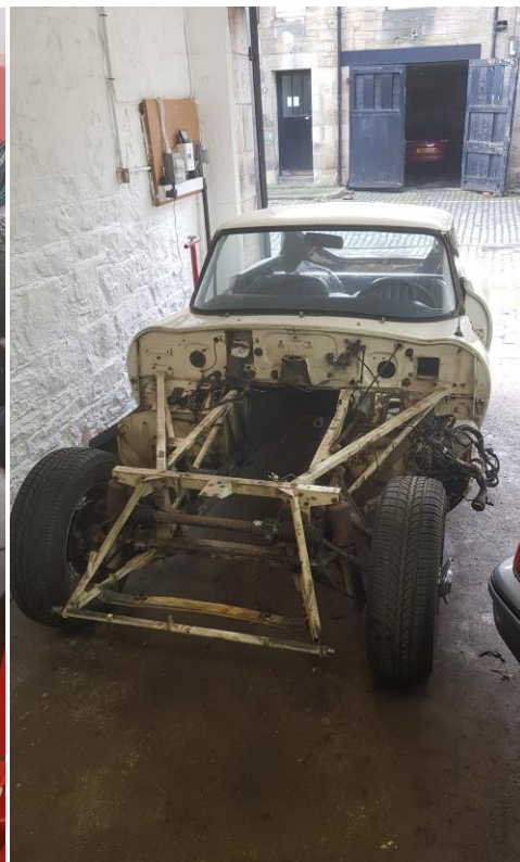
Engine removal – simpler at this stage to lift the car over the engine rather than engine over the car
