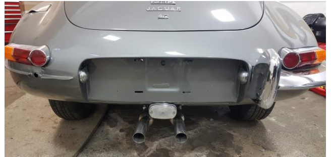
A gorgeous new stainless steel sports exhaust system from manifold back was fitted (note IRS had yet to be restored at this stage)
