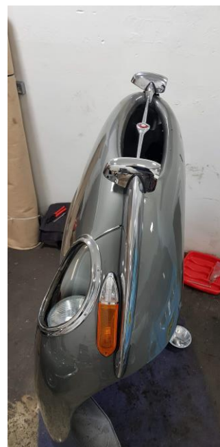
UK RHD headlights and bumper chromes fitted, without US bull bar
