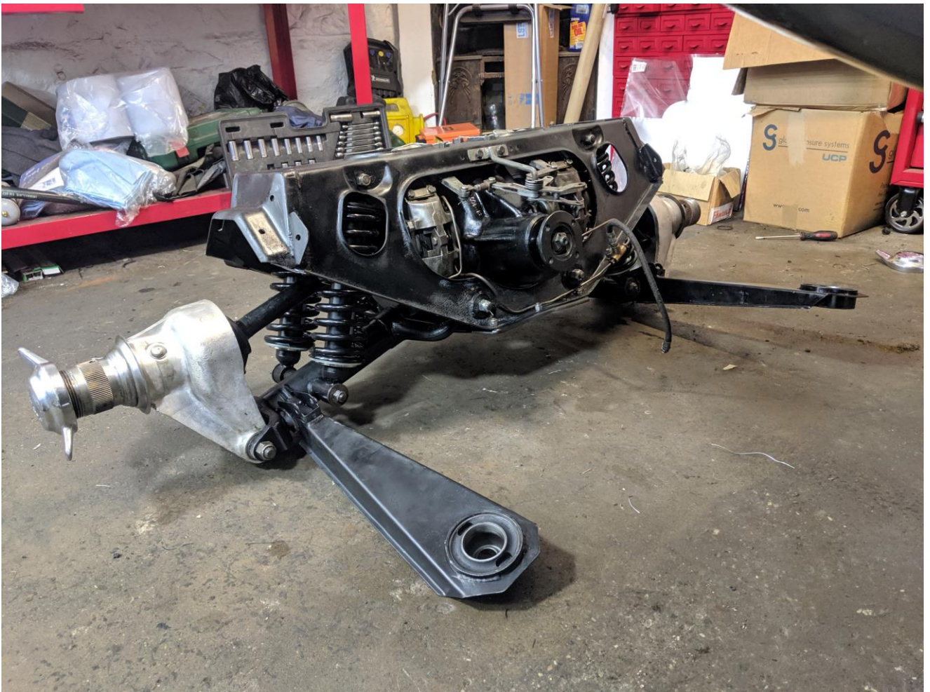
Completed IRS ready for installation, with brand new bushes, shocks and springs throughout. Notice the inboard disc brakes.
