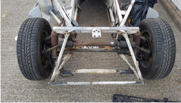
Final strip-down and treatment of surface rust prior to delivery of body to a specialist paint company
