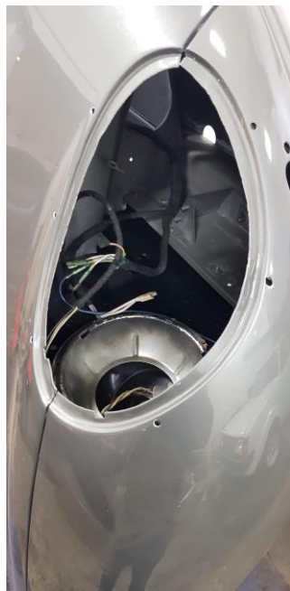
Front lights were rewired and the base plates painted
