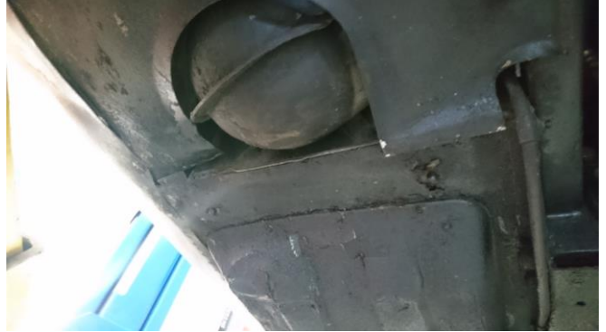
LHD cars have brake master cylinder, servo and fluids near exhaust on an asbestos board – this will need to be changed
