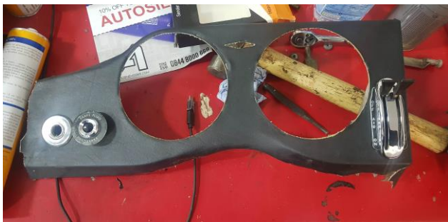
Left-hand drive clocks restored then changed to right-hand drive
