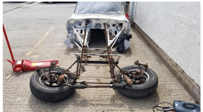
Final strip-down and treatment of surface rust prior to delivery of body to a specialist paint company
