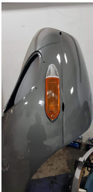
US indicators removed, with UK indicators being fitted
