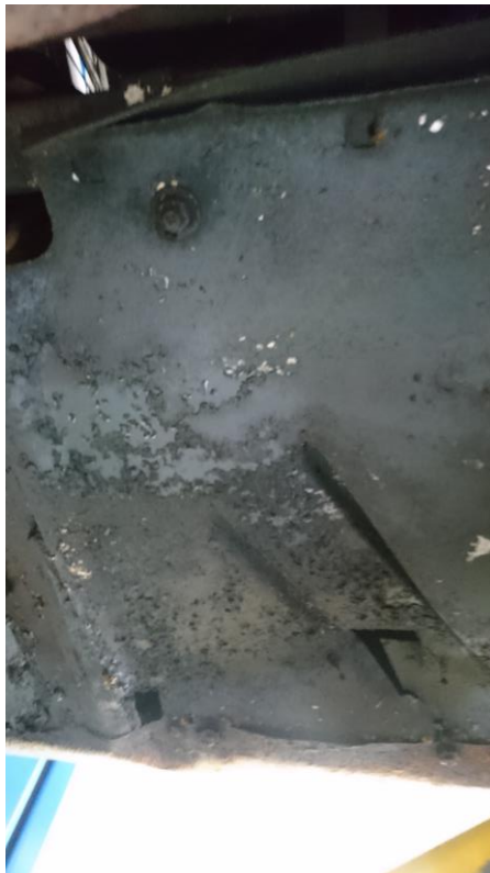
LHD cars have brake master cylinder, servo and fluids near exhaust on an asbestos board – this will need to be changed
