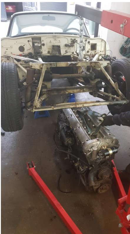
Engine removal – simpler at this stage to lift the car over the engine rather than engine over the car
