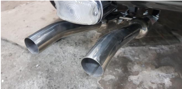
A gorgeous new stainless steel sports exhaust system from manifold back was fitted (note IRS had yet to be restored at this stage)
