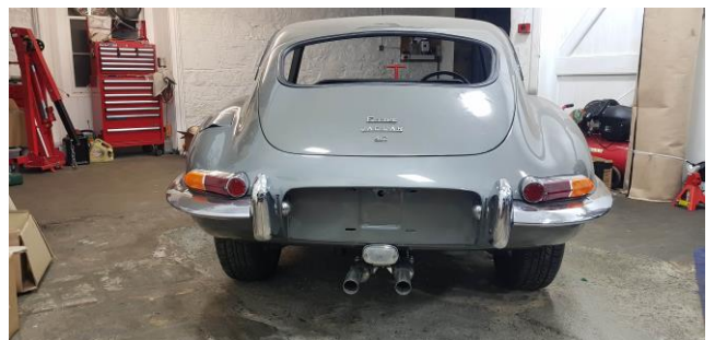
US rear bull bars were removed from the bumper chromes
