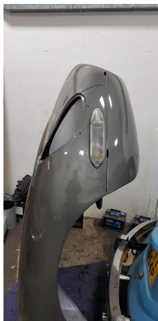
US indicators removed, with UK indicators being fitted
