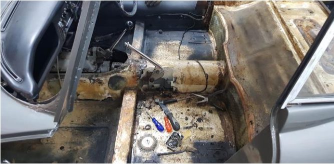
Floor being treated prior to sound deadening installation
