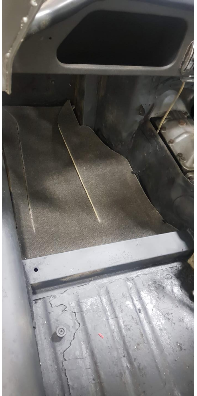
New underlay being applied to the black treated sound deadening
