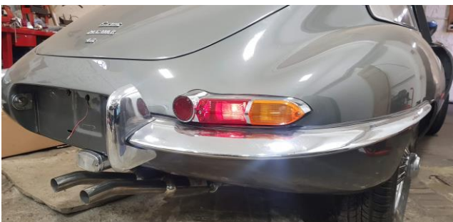
UK rear lights were sourced and installed
