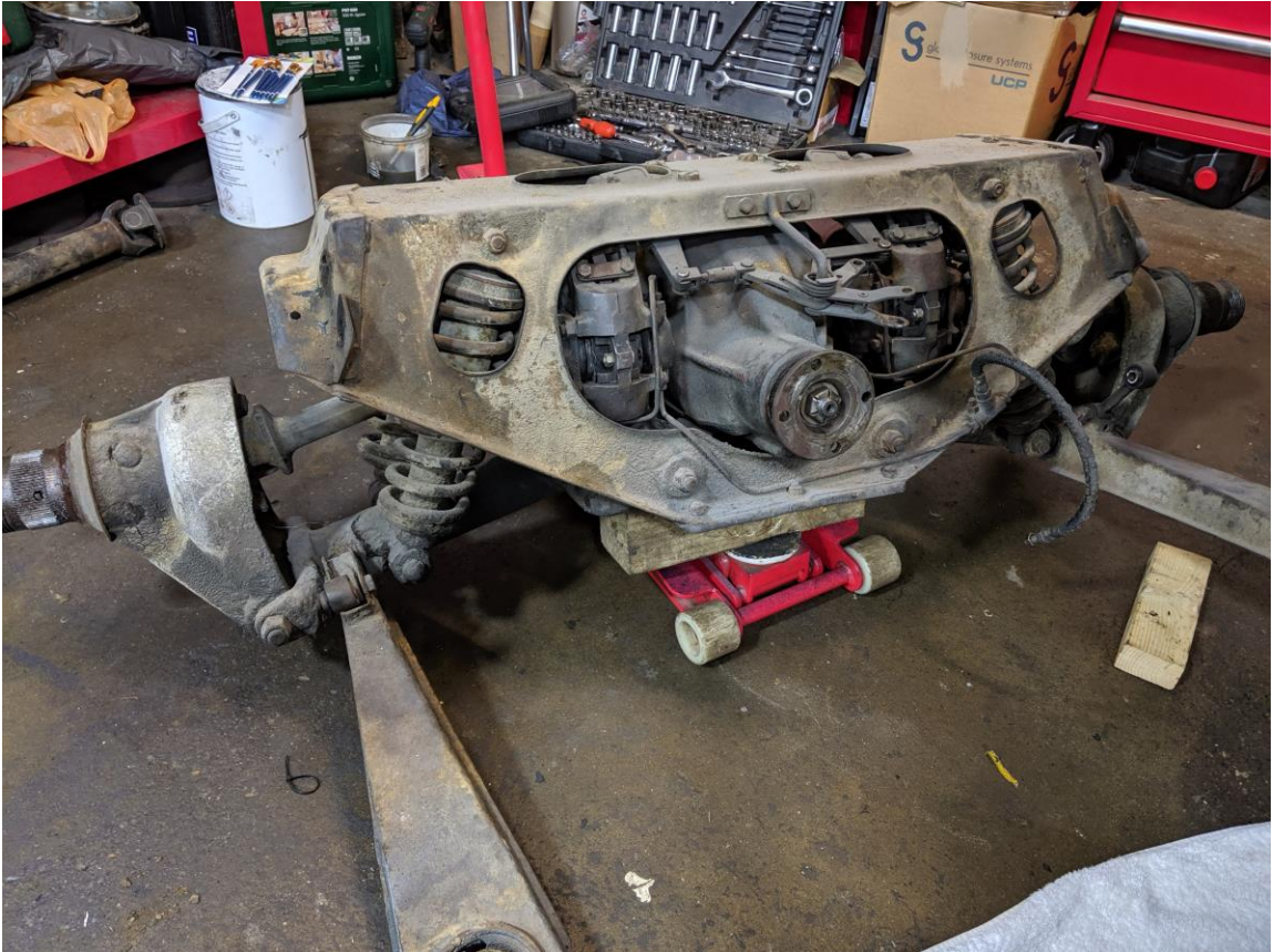
IRS dropped from car for nut and bolt rebuild
