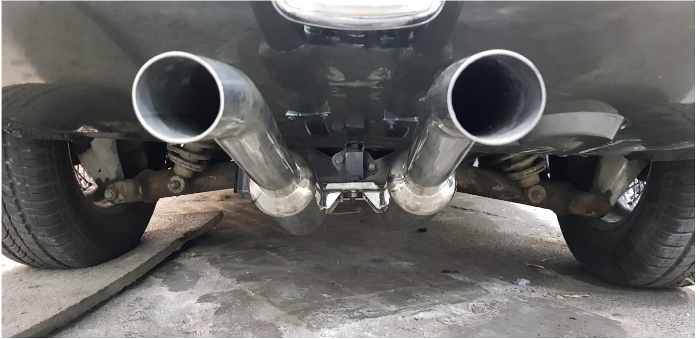
A gorgeous new stainless steel sports exhaust system from manifold back was fitted (note IRS had yet to be restored at this stage)
