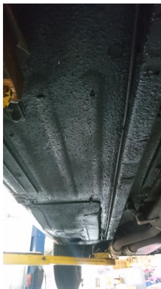
Underside of chassis rust free
