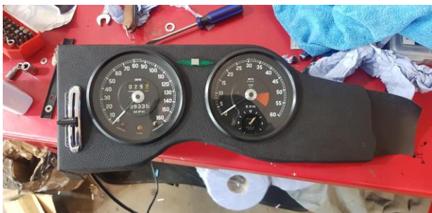
Left-hand drive clocks restored then changed to right-hand drive
