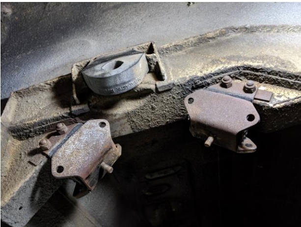
Bushes on the chassis were also replaced – these old ones were in good shape but were changed regardless
