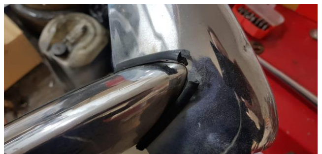
New bumper trim strips fitted to replace the old broken ones
