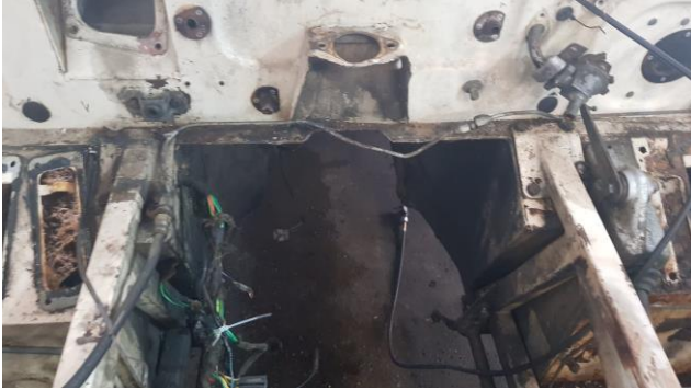
Final strip-down and treatment of surface rust prior to delivery of body to a specialist paint company
