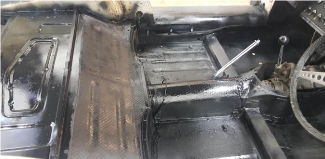
Floor being treated prior to sound deadening installation
