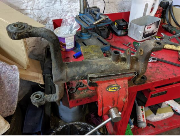
One of the wishbones being dismantled
