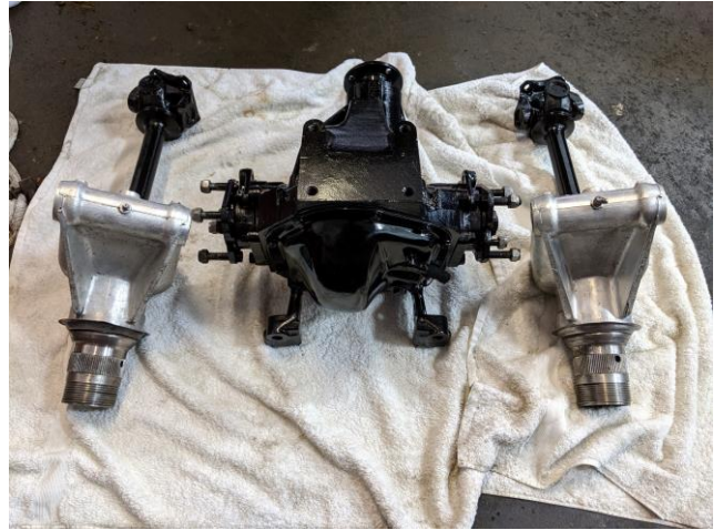
Differential and driveshafts rebuilt
