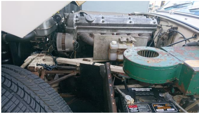
LHD cars have brake master cylinder, servo and fluids near exhaust on an asbestos board – this will need to be changed
