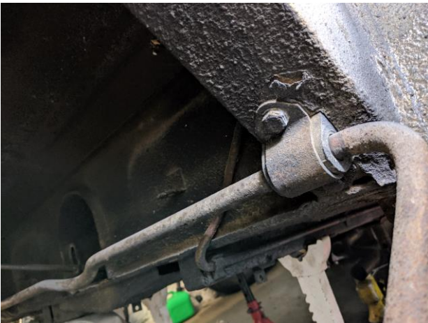
Bushes on the chassis were also replaced – these old ones were in good shape but were changed regardless
