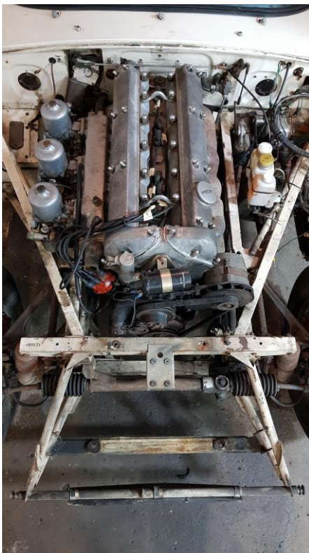
Asbestos shielding, between exhaust and brake fluid, flaking off
