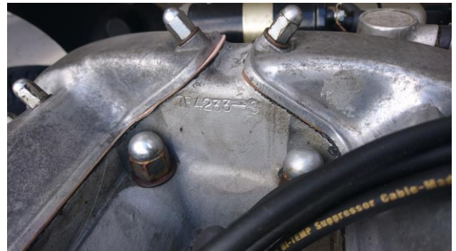
Cylinder head 7F4233 indicating replacement head
