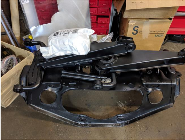
IRS carriage and wishbones back from powder coating
