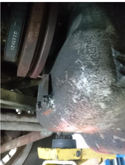
Rope seal on crank is notorious for leaks – this one is sound
