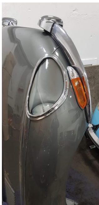
UK RHD headlights and bumper chromes fitted, without US bull bar
