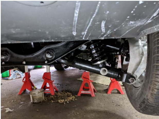
Rear suspension reinstalled on the car
