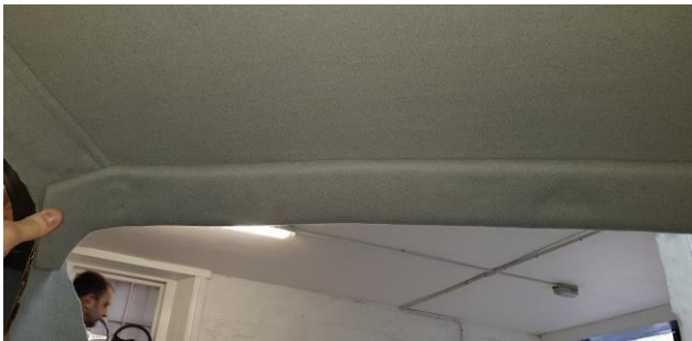
Headlining edge finishing being installed
