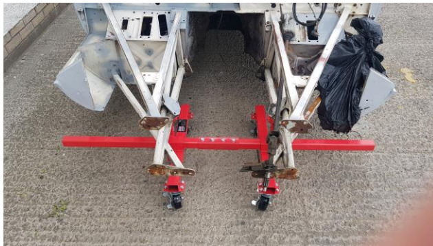
Use of one of Investor Classics' chassis dollies to manoeuvre the chassis without front wheels
